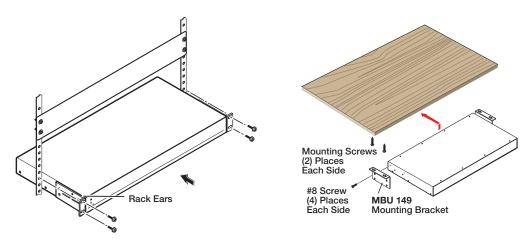
Figure 2. Mounting the Annotator 300; rack or under-desk mounting.
